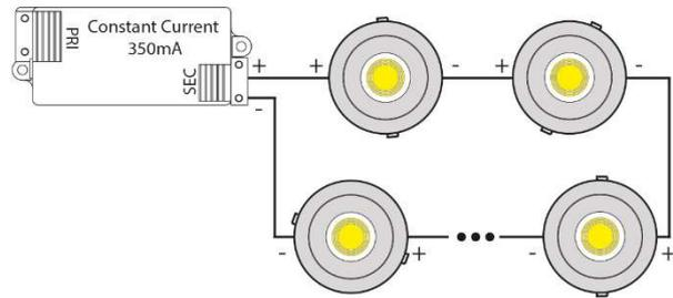
\*Do not connect the luminaire to an active LED driver. Some LED drivers emit high voltage when idle, which may cause permanent damage to the luminaire. Be sure to disconnect the LED driver from the power line before connecting the luminaire.
